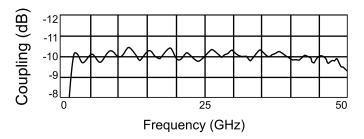
(Figure 1) Coupling characteristics of Krytar Model 102050010
